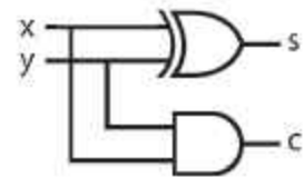
Figure 3.16: Truth table and required circuit for a Half Adder
